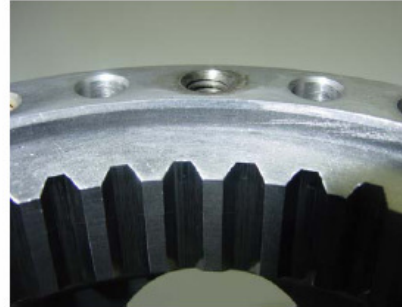
CHAMFERED FACE ON END OF SPLINES
