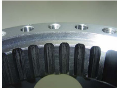
SQUARE FACE ON END OF SPLINES
